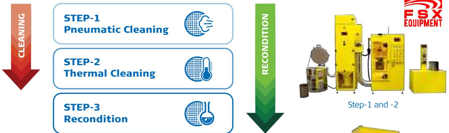
Normal cleaning includes only step-1 and step-2 using pneumatic and thermal cleaning to remove loose ash and to partly remove hardened ash.
